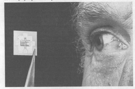
CLOSE EYE on an interfacial force sensor: The developer of the sensor, Jack Houston (1114), holds an example in forceps to display its relative size.
